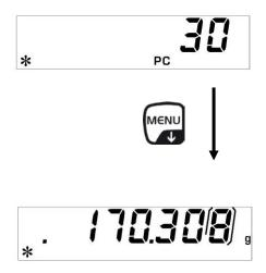
⇒ Press **MENU** button, the total weight of the placed parts is displayed.
